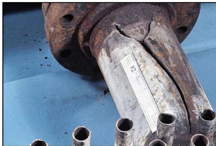
**Figure 7: Post Incident photograph of liquid transfer vessel with insulation removed.**
