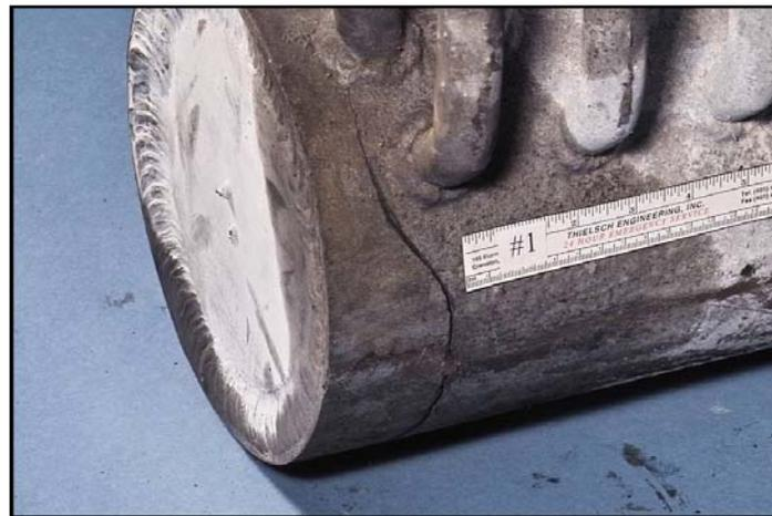
**Figure 5: Close-up photographs of cracking adjacent to right end plate of suction header #1.**
